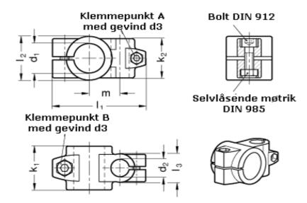
Adjustable clamp lever for d3 = GN 911-M10-55 have to be ordred separately Adjustable clamp lever for d4 = GN 911-M 8-32 have to be ordred separately d1 = 45 d2 = 30 d3 = M10 d4 = M8 k1 = 65
